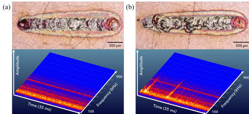
Fig. 1. (a) Picture of a good weld seam with the spectrogram of its acoustic emissions; (b) Picture and spectrogram of a faulty weld seam
