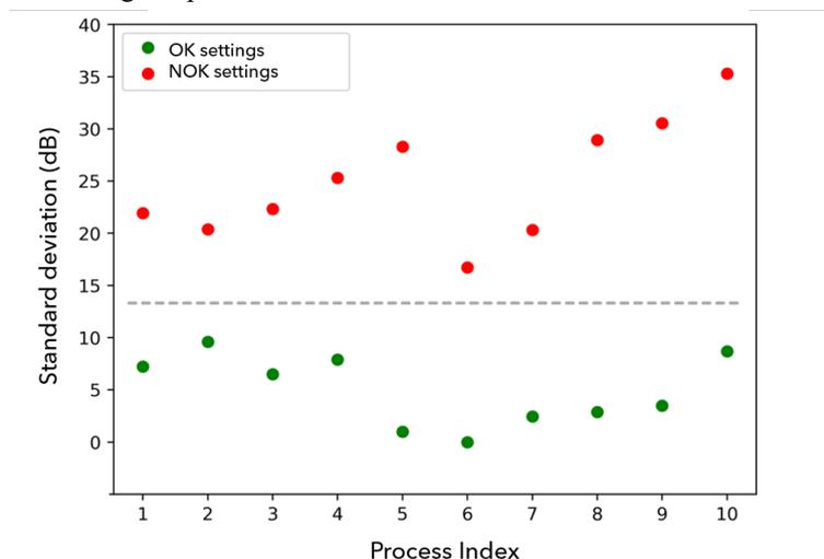
Fig. 2. Diagram of the standard deviations of the acoustic energies emitted by welding processes with good settings (marked in green) and with faulty settings (marked in red)
