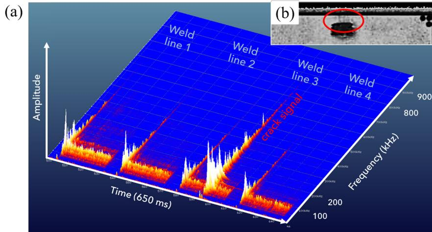
Fig. 3. (a) Spectrogram of four welding processes with a crack due to thermo-shock appearing during the third weld seam. This defect produces a high-amplitude and very broadband acoustic signal. (b) Microscope image of the crack (in red circle) in the ceramic due to thermo-shock
