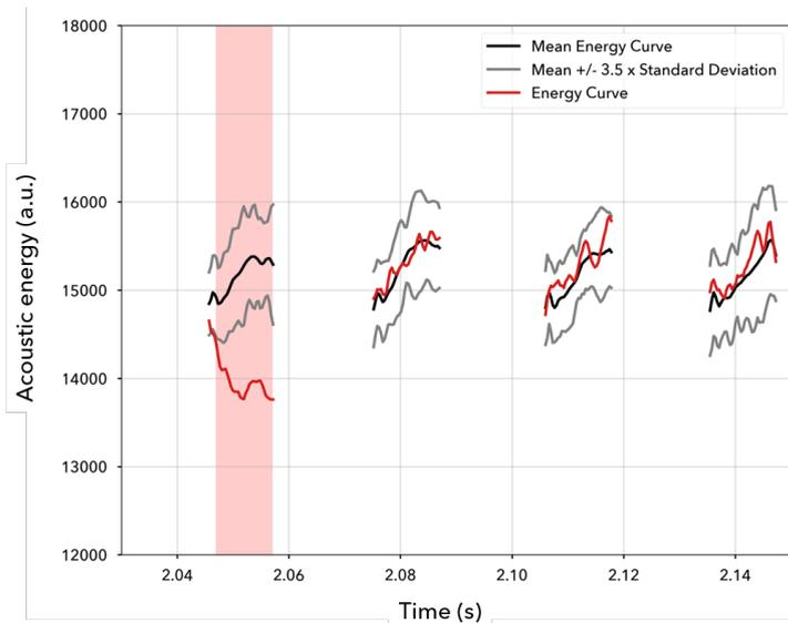
Fig. 4. Diagram of an envelope analysis on the misalignment of weld seams. The first one contains the defect (misalignment), while the other three are flawless.
