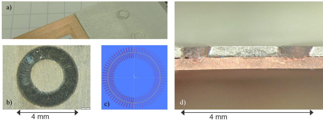
Fig. 2. Wobble welding of Al on Cu a) b) overview and detail of welding from top side c) wobble geometry d) cross section through ring center
