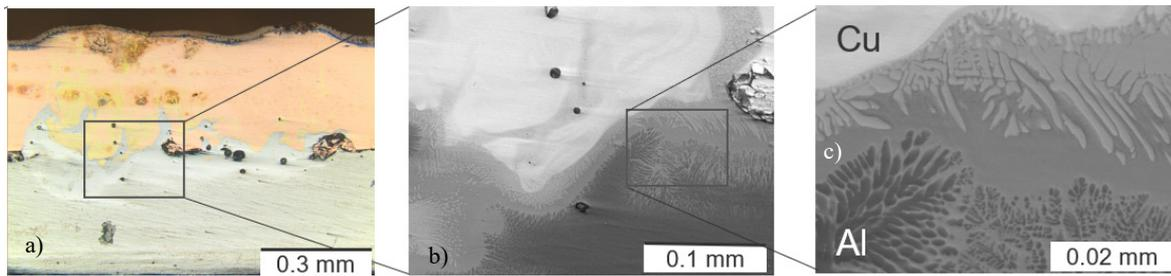
Fig. 4. Hatch welding of Cu on Al, cross section, a) microscopic image b) c) SEM image
