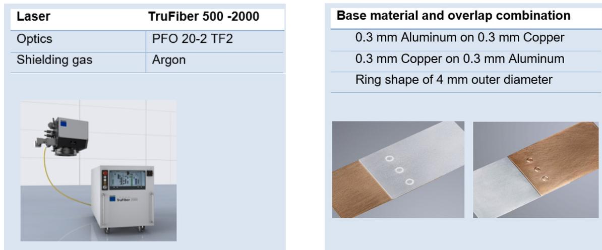
Fig. 1. Laser, optical setup and workpiece combinations
