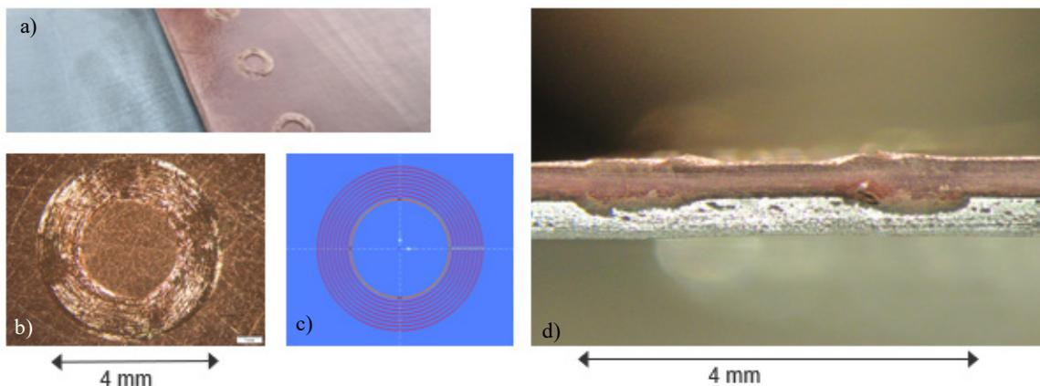
Fig. 3. Hatch welding of Cu on Al a) b) overview and detail of welding from top side c) hatch geometry d) cross section through ring center
