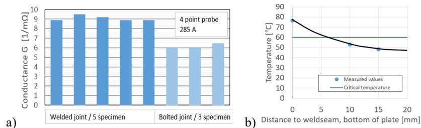
Fig. 5. a) Electrical test of the Cu-Al connection. Comparison of the conductance between joints realized with hatch welding (left) and bolted connections (right), b) Temperature measurements during laser hatching process as function of the distance from the center of the ring.
