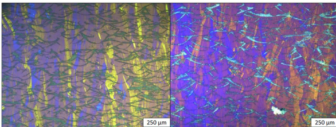
Fig. 4. Metallographic inspection perpendicular to build direction of AlCrSc in polarized light – Baker’s etch depicting large columnar grains
