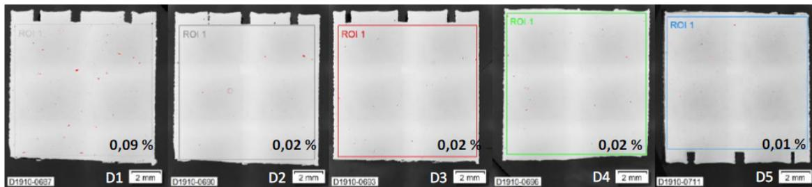
Fig. 2. LPB-F “density cubes” of LPB-F processed AlCrSc with different LPB-F process parameter
