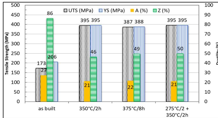
Fig. 3. Static strength values of AlCrSc alloy in the “as built state” & annealed 350°C/2 – 375°C/8h – 275°C/2h + 350°C/2h
