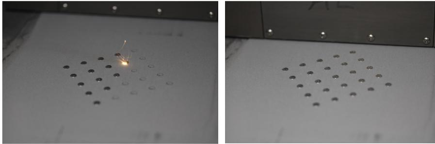
Fig. 1. AlCrSc alloy during LPB-F processing (no “smoke” evolution &amp; reduced spatter) &amp; after processing (“stainless steel look”)
