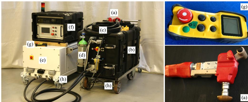
Fig. 2. Laser system for mobile outdoor material processing (laser rescue activities), consisting of handheld laser processing device (a), fiber laser source implemented into an outdoor box according to military standards (b), protected fiber-optic cable (c), process gas supply via breathing air cylinder (d), cooling unit (e), laser safety control unit (f), remote control (g) and transport trolleys (h).
