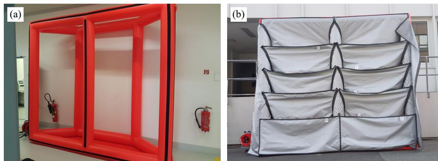
Fig. 3. Concept of an inflatable framework structure (a) covered with laser-protective curtain elements (b) to set up a laser area.
