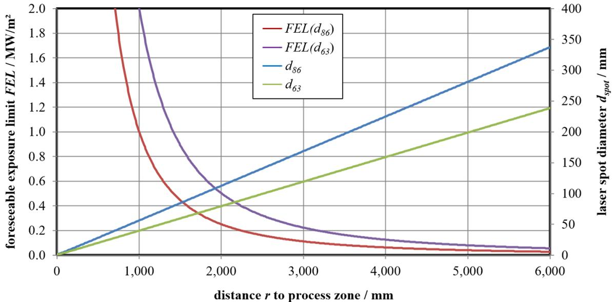
Fig. 1. Foreseeable exposure limits  $FEL(d_{86})$  and  $FEL(d_{63})$  and corresponding laser spot diameters  $d_{86}$  and  $d_{63}$  as a function of the distance  $r$  to the laser process zone. Further explanations are given in the text.
