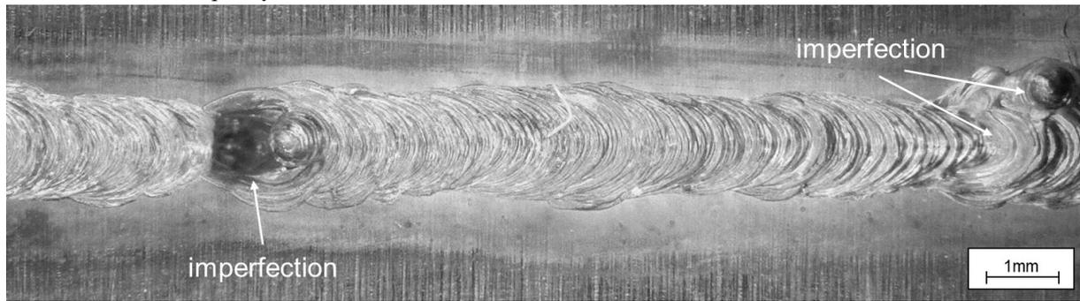
Fig. 5. Reference process,  $v = 6$  m/min, weld surface.
