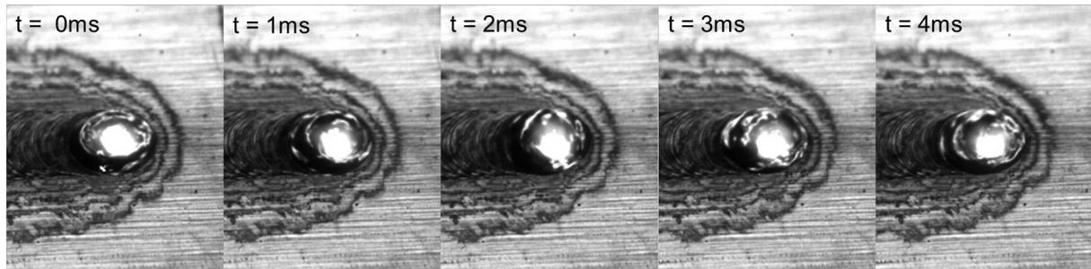
Fig. 7. ARM laser,  $v = 3$  m/min, process observation using high speed camera.
