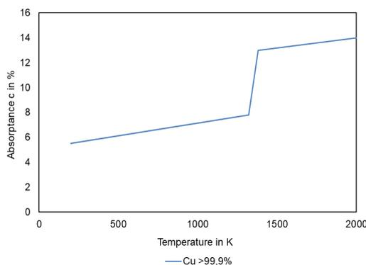
Fig. 1. Temperature depended Absorption for a wavelength of 1  $\mu\text{m}$ , Engler (2015), Blom et al. (2003).
