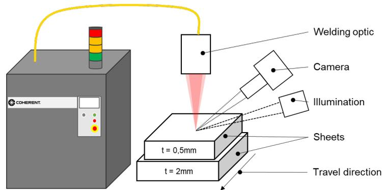
Fig. 3. Schematic experimental setup.
