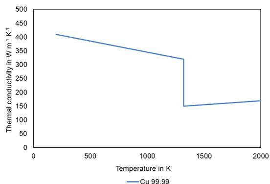
Fig. 2. Thermal conductivity of Cu, Cargan (2010), Pottlacher (1999).
