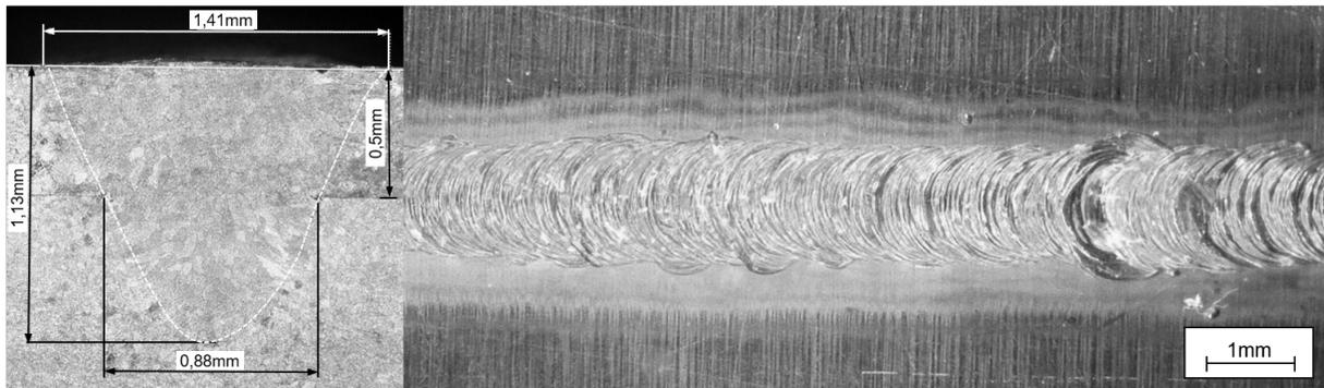
Fig. 6. ARM laser,  $v = 5$  m/min, cross section and weld surface.
