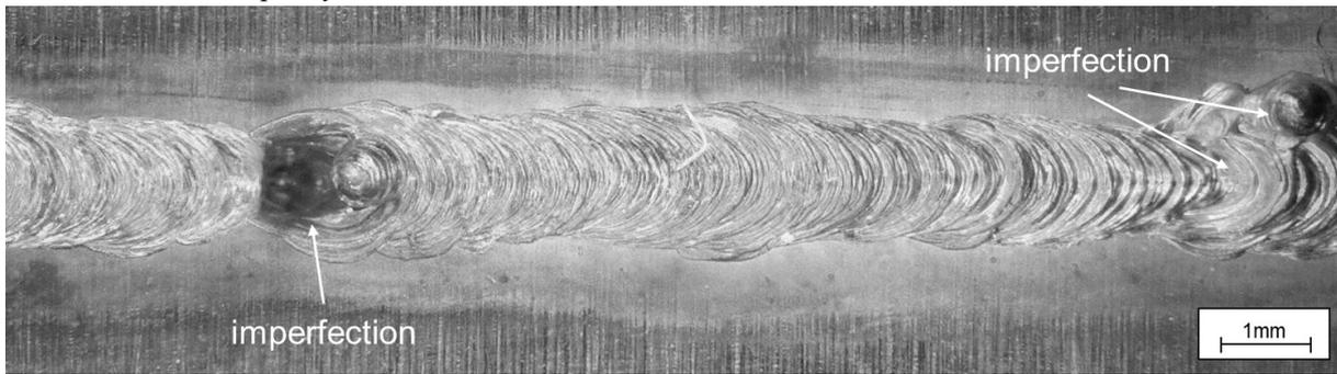
Fig. 5. Reference process,  $v = 6$  m/min, weld surface.
