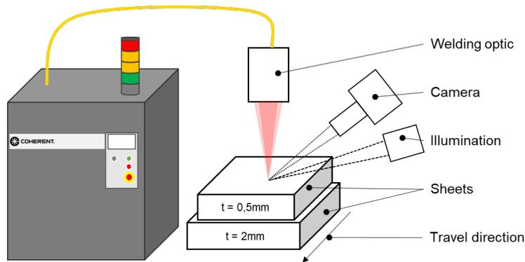
Fig. 3. Schematic experimental setup.
