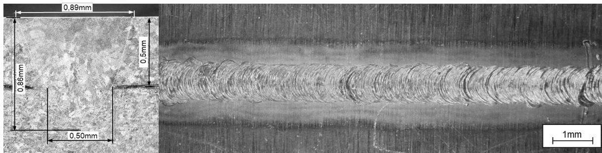
Fig. 8. ARM laser,  $v = 3$  m/min, cross section and weld surface.
