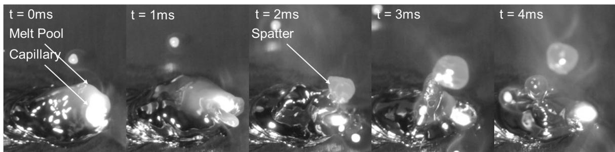
Fig. 4. Reference process,  $v = 6 \text{ m/min}$ , process observation using high speed camera.
