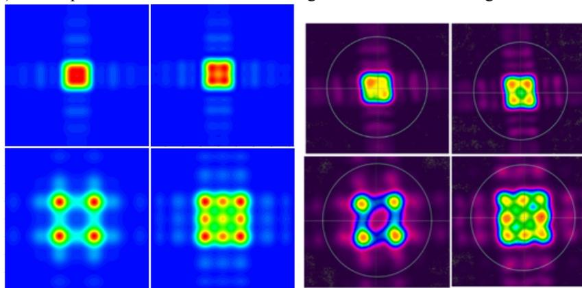
Fig. 2. (left) Simulated intensity profiles in the focal region of a lens as in Fig. 1 employing a freeform optical phase plate; (right) Corresponding measured intensity profiles. The dimension of the profiles depend on the NA of the focusing lens and usually range from  $20\mu\text{m}$  to  $500\mu\text{m}$ .
