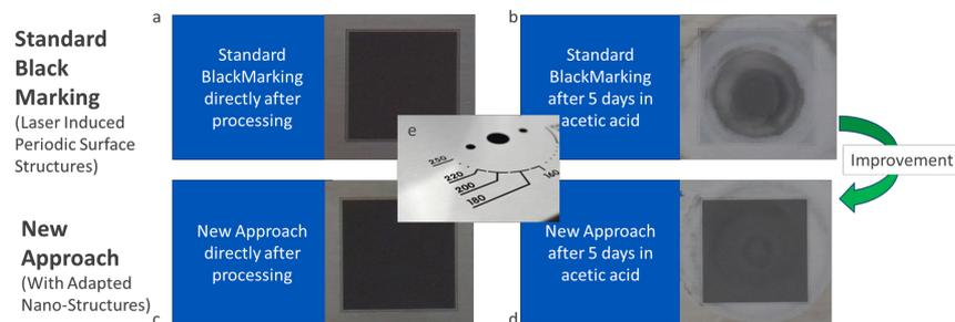
Fig. 7. Achieved improvement due to simulation-based process development (e.g. for the black-marking of household [white] goods like shown in sub-figure e)
