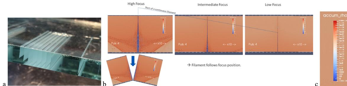
Fig. 1. (a) Filament curtain inside a glass bulk volume (b) Simulation of bulk ionization inside the glass material for filament cutting (pseudo-color shows electron density and thus damage (in red) as well as void formation (in blue)); the change of the filament structure due to a change in focal position is shown in the different pictures from left to right where the working distance is continuously decreased (c) common logarithmic legend of the accumulated electron density in  $1/\text{cm}^3$
