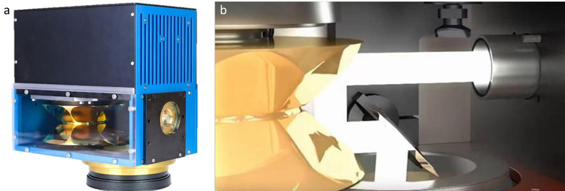
Fig. 1. (a) Compact polygon mirror scanner of the “PM series” from MOEWE and (b) detailed visualization of the laser beam propagation inside the scanner reflecting the laser light three times.
