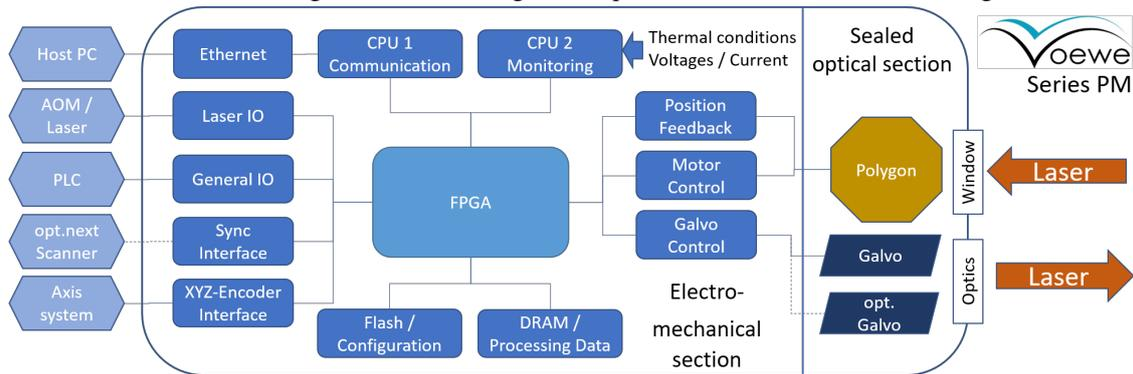
Fig. 2. Overview of the network within the fully digital controlling unit based on a FPGA
