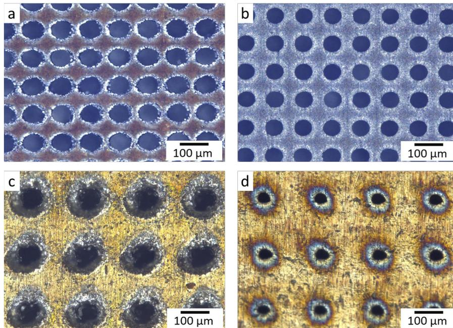
Fig. 3. High speed drilled holes in silicon wafers front side (a), back side (b) with a spacing of  $100\ \mu\text{m} \times 100\ \mu\text{m}$  using 30 pulses and drilled stainless steel front side (c), back side (d) with a hole spacing of  $200\ \mu\text{m} \times 200\ \mu\text{m}$  using 120 pulses
