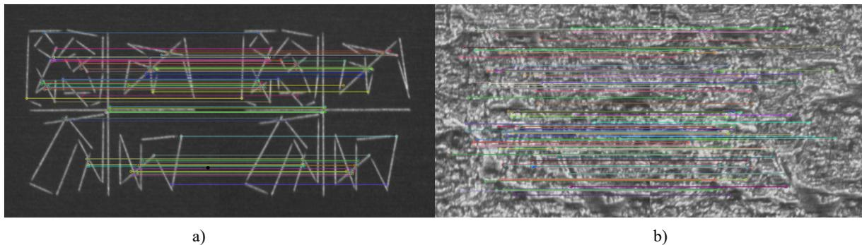
Fig. 2. calculated displacement vector for (a) a marker and (b) the texture itself.
