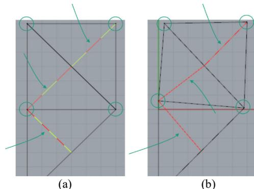
Fig. 3. (a) Pre-calculated toolpath consisting of a simple line crossing intersections of segments. (b) Adapted toolpath regarding the measured displacement vectors.
