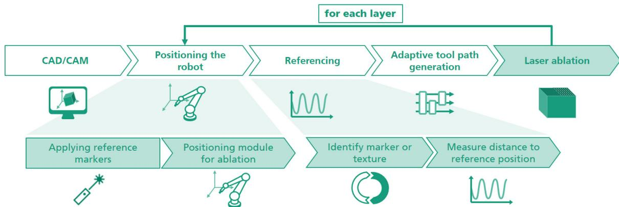
Fig. 1. Process chain for robot based laser structuring.
