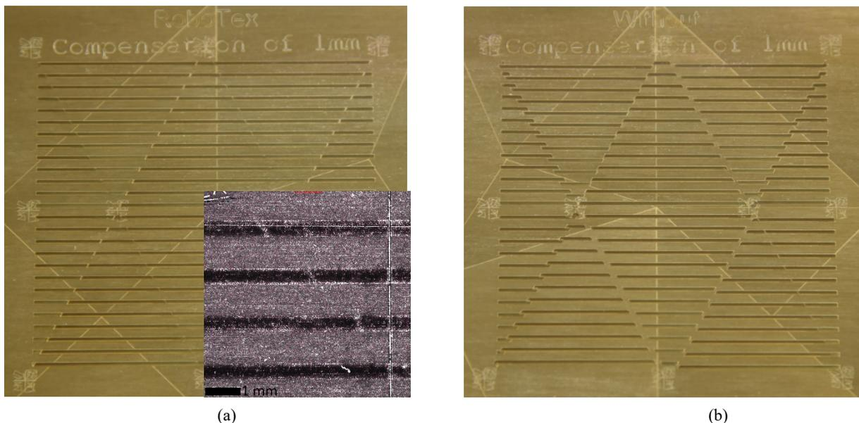
Fig. 5. (a) Resulting surface applying the compensation strategy to a random position uncertainty of 1 mm. (b) Resulting surface with the same setting but compensation method switched off.
