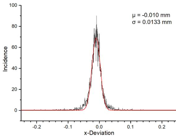
Fig. 4. x-value of the displacement vector for  $n=5000$  images of one marker.
