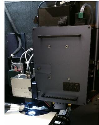
Fig. 1. FlexibleBeamShaper integrated in a laser machine configuration with a femtosecond laser system
