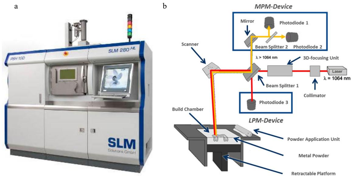
Fig. 1. (a) SLM 280<sup>HL</sup>; (b) Schematic assembly of optic design with Melt Pool Monitoring and Laser Power Monitoring.
