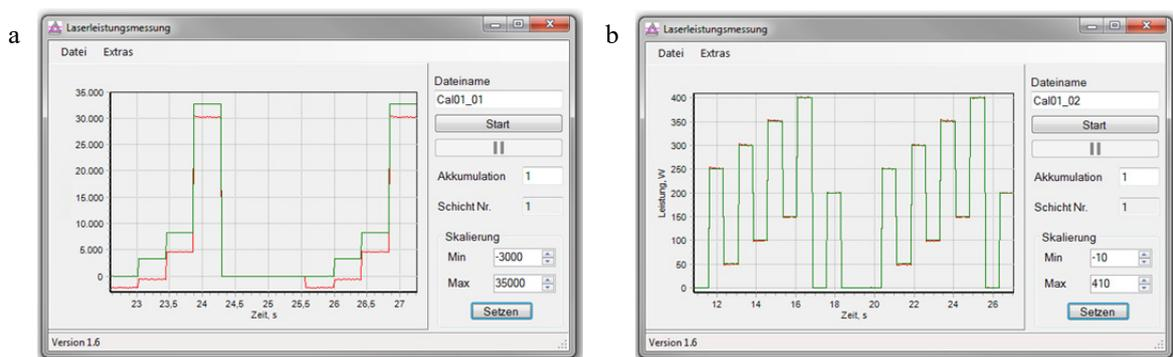
Fig. 3. (a) Adjustment for set and measured laser power; (b) Calibration rechecks for laser power adjustment up to 400 W.
