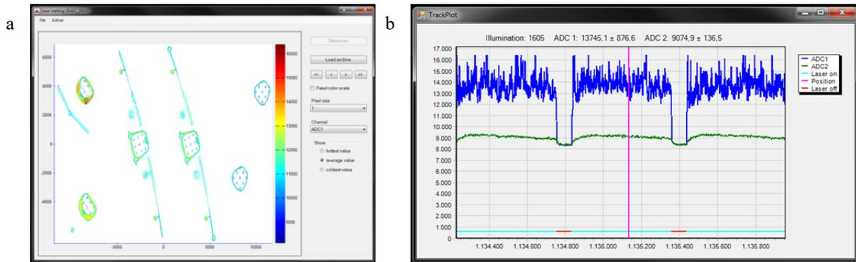
Fig. 2. (a) Layerwise x/y 2D representation of thermal emissions; (b) Complementary Track Plot of selected scan vector.
