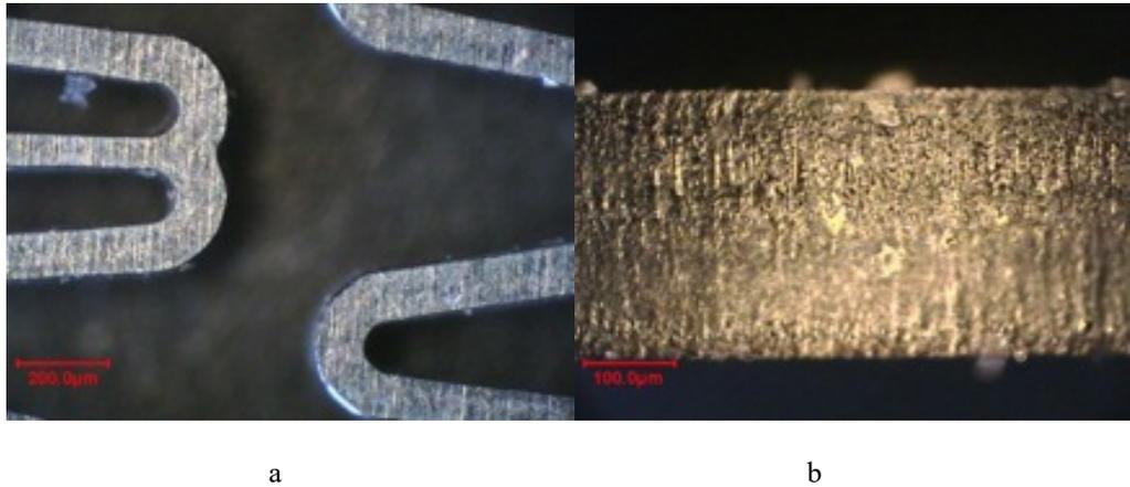
Fig. 3. Stainless steel sheet cut sample (a) top view (b) side view.
