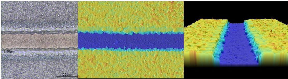
Fig. 5. Optical and confocal microscopic appearance of the P3 structuring result with fs laser pulses and flattop beam profile.
