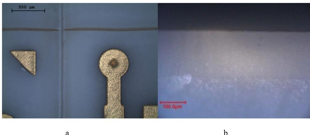
Fig. 2. Silicone film on ceramic substrate (a) top view laser cut in silicone (b) cut and broken ceramic sidewall.
