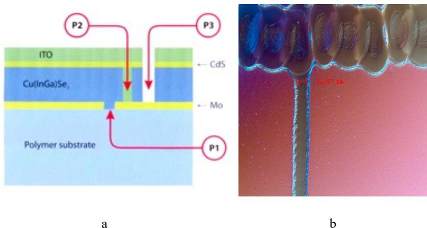
Fig. 4. P1, P2 and P3 structuring process (a) process steps (b) P1 structuring with fiber laser and ultra short pulse laser.
