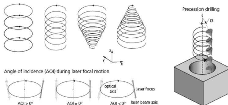
Fig. 2. System design for flexible laser processing in the  $\mu\text{m}$  range.
