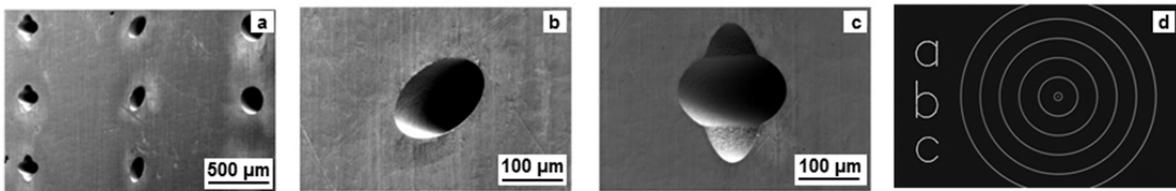
Fig. 6. (a) Flexible geometries in 300- $\mu$ m-thick steel; Details of figure (a): (b) Elliptical bore hole (190  $\mu$ m long, 110  $\mu$ m wide); (c) Geometric flexibility achieved by two overlapping ellipses; (d) Marking pattern for labeling – 0.5 mm font size, font type SimpleStraight3.
