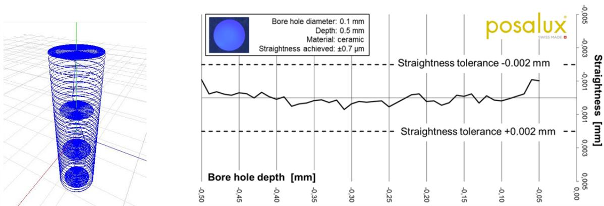
Fig. 5. Visualization of the 3D laser focal motion path in precSYS's software DrillControl (left), Measuring report for a 100- $\mu$ m-bore hole generated with a precSYS in 500  $\mu$ m thick ceramic (right) - provided by Posalux SA.
