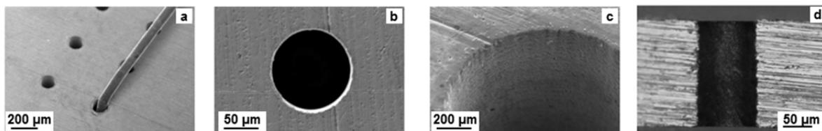
Fig. 4. (a) 100- $\mu\text{m}$  bore hole array in steel (entrance side) compared to a human hair; (b), (c) single bore hole from (a) magnified; (d) cross section of a  $0^\circ$  taper 100- $\mu\text{m}$ -bore hole in 200- $\mu\text{m}$ -thick steel (process time  $\sim 1\text{s}$ ).
