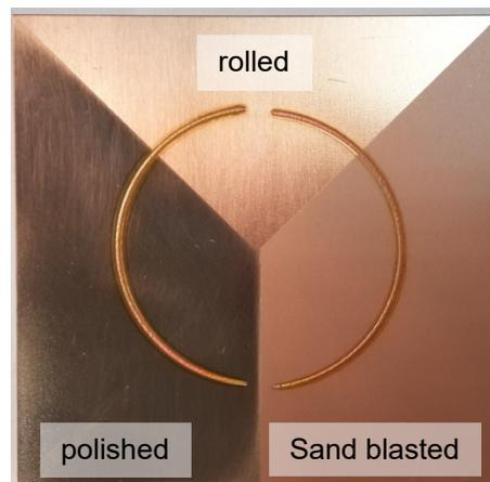
Fig. 3. Excellent weld seams at different material surface.
