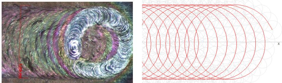
Fig. 1. Feed rate: 10 mm/s; Radius 0,5 mm; Freq.: 100 Hz.
