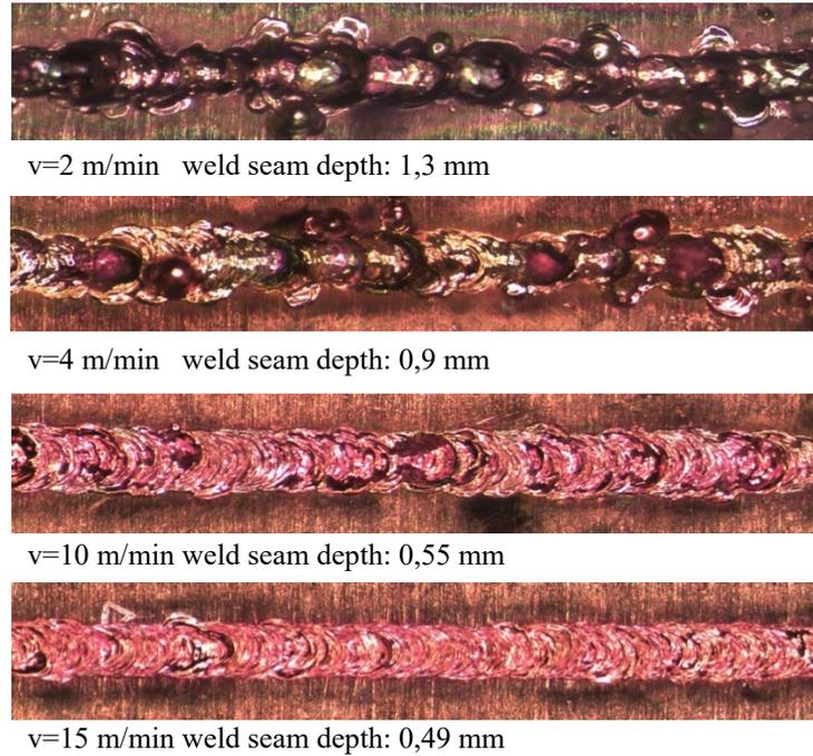
Fig. 1. Weld seams at different speeds and Power of 1,5kW.
