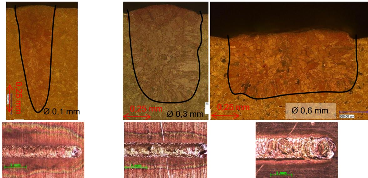
Fig. 2. Weld seams with variable wobbling diameter, Power: 1kW, 1m/min, 300Hz.
