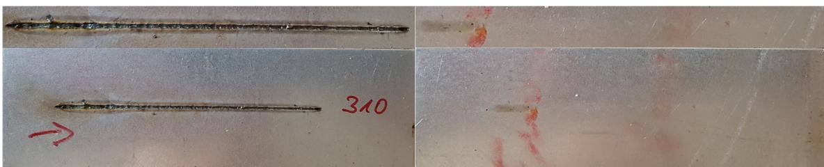
Fig. 7. Top- and backside of the depth controlled weld.
