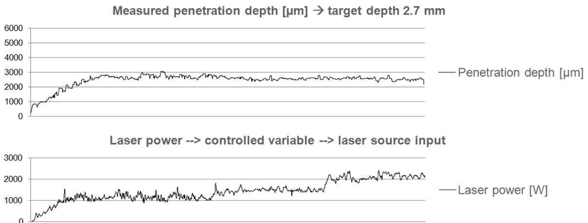
Fig. 6. Measured penetration depth (top) and control signal to the laser source (bottom).
