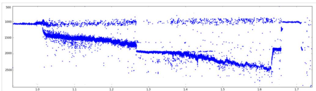
Fig. 3. Raw signals of the measuring system during welding of an overlap weld joint applying a power ramp.
