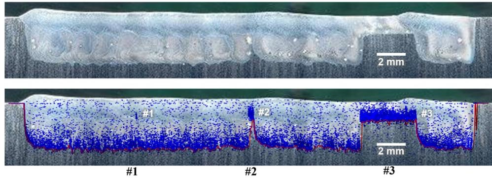
Fig. 4. Example: automated signal extraction for a weld stainless steel and three intentional interruptions of the laser power (#1: 1 ms; #2: 10 ms; #3: 100 ms).
