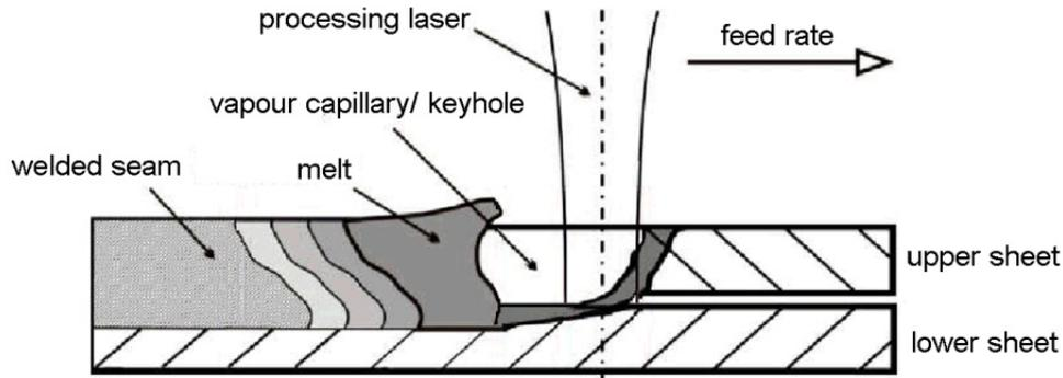
Fig. 2. Schematic figure of an overlap weld joint configuration with gap.
