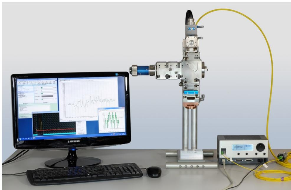
Fig. 8. IDM sensor system adapted to a commercially available laser welding head.
