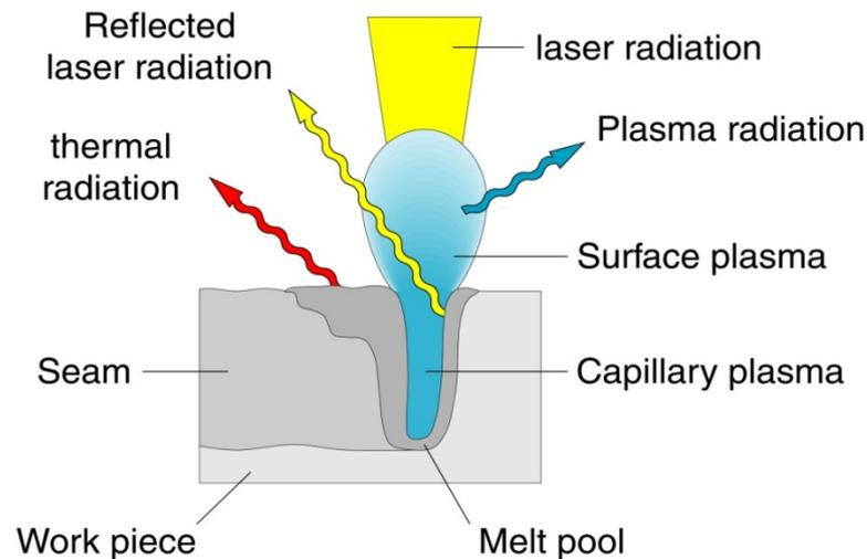
Fig. 1. Overview of the electromagnetic emissions during laser beam welding.
