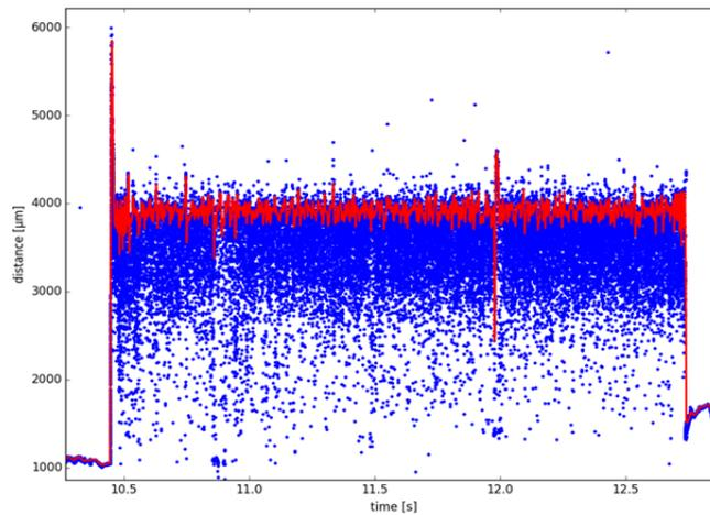
Fig. 5. Controlled process: Setpoint 3 mm penetration depth.
