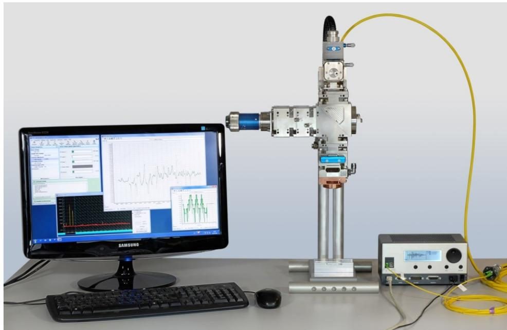
Fig. 8. IDM sensor system adapted to a commercially available laser welding head.
