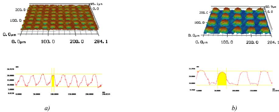
Fig. 1. (a) master structure (stainless steel) generated by laser ablation (b) replication by injection molding (PLGA)
