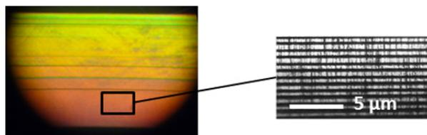
Fig. 3. Laser-ablated microgrooves in the sub-micrometre range on a curved surface acting as a diffraction grating with iridescent reflections.
