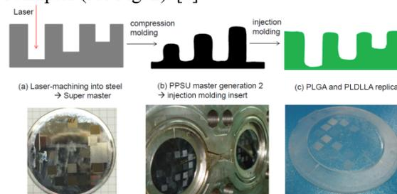
Fig. 2. Scheme of the process chain used for injection molding of PLGA substrates with a panel of different cell-harboring micro-well structures. The depicted PLGA sample (lower right) has a diameter of 6.5 cm.
