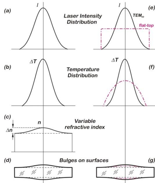
Fig. 1 Effects by gradient heating of a protective window.
