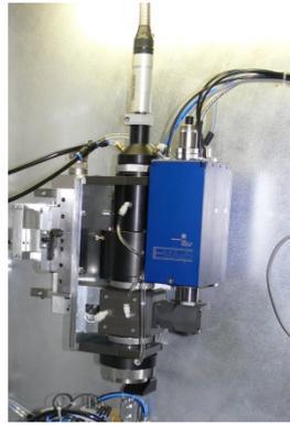
Fig. 6. »E-MAqS« with aluminum housing mounted to an optics of a high power diode laser for coaxial measurement.
