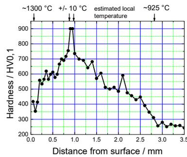
Fig. 1. Hardness over penetration at a laser heat treated surface, pre-heated part made of X155CrVMo12.1, temperature gradient estimated from experimental data of heat treated samples.
