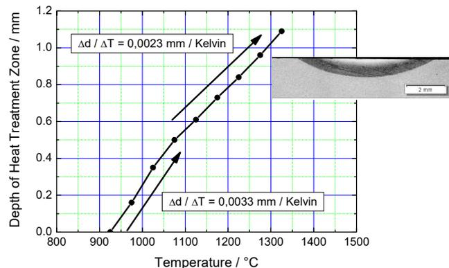
Fig. 2. Depth of the hardening zone (d) in dependence of the surface temperature (T), flat samples made of tool steel X155CrMoV12.1, depth was measured in the etched cross section (example at top of diagram).
