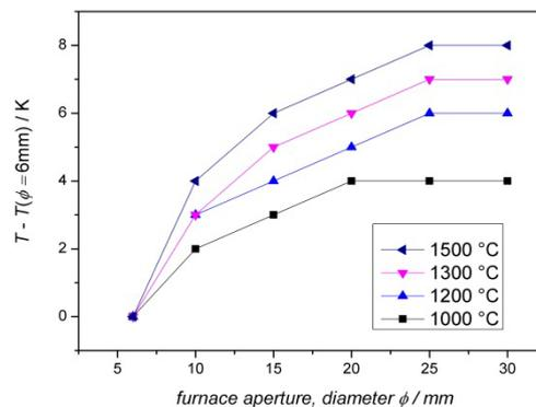
Fig. 4. Influence of the size-of-source effect (SSE) on the temperature characteristics of a thermal imaging system based on a CCD camera.
