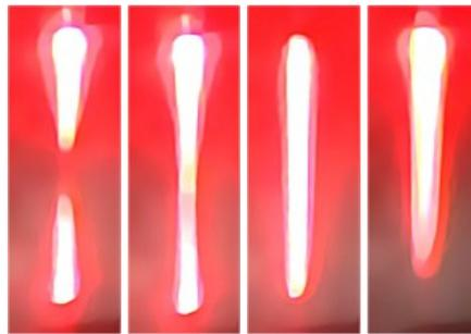
Fig. 9. Laser power density distribution, detected with special infrared camera (spot size: about 6 x 80 mm<sup>2</sup>), optimization via scanning function.
