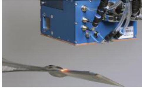
Fig. 8. »LASSY« at turbine blade hardening.
