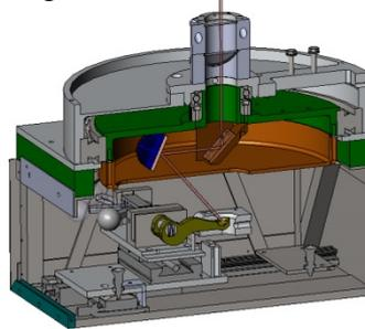
Fig. 14. Rotating mirror device for laser hardening of brake levers.
