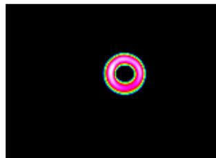
Fig. 10. Temperature dispersion during a typical laser hardening process of a valve seat like Figure 11, measured with »E-MAqS« camera system coaxial thru the laser optics with ring shaped laser spot.
