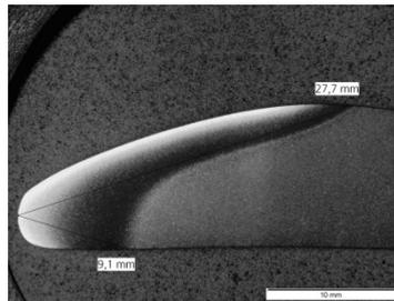
Fig. 12. Typical cross section of a laser hardened turbine blade.
