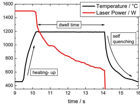
Fig. 3. Process data of a temperature controlled laser heat treatment process of the end face of a screw, temperature measured with pyrometer MAURER KTR 1075.
