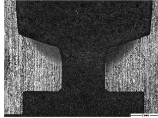
Fig. 11. Cross section of a laser beam hardened valve seat.
