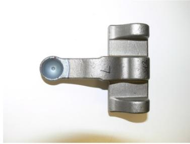
Fig. 13. Brake lever, laser beam hardened in as-forged state.
