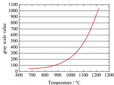
Fig. 5. Typical dependency of grey scale values on the surface temperature at given attenuation, filter set and shutter adjustment.
