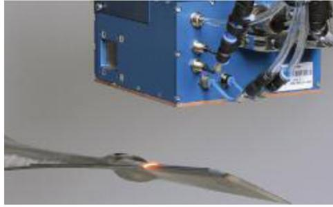
Fig. 8. »LASSY« at turbine blade hardening.
