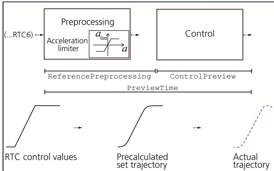
Fig. 1. Structure of *SCANAhead* servo control.
