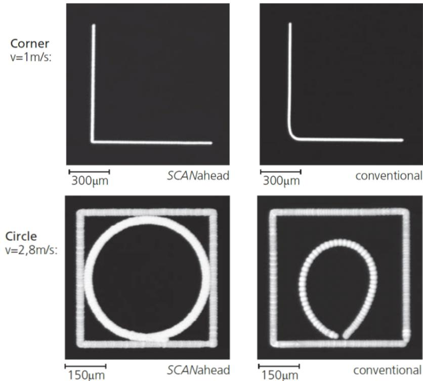
Fig. 4. Marking results illustration the differences between conventional control and *SCANahead* control.
