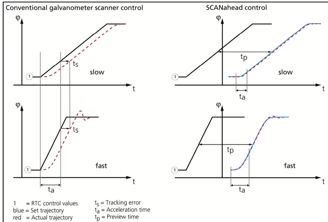
Fig. 2. Comparison: Conventional galvanometer scanner servo control and SCANahead servo control.
