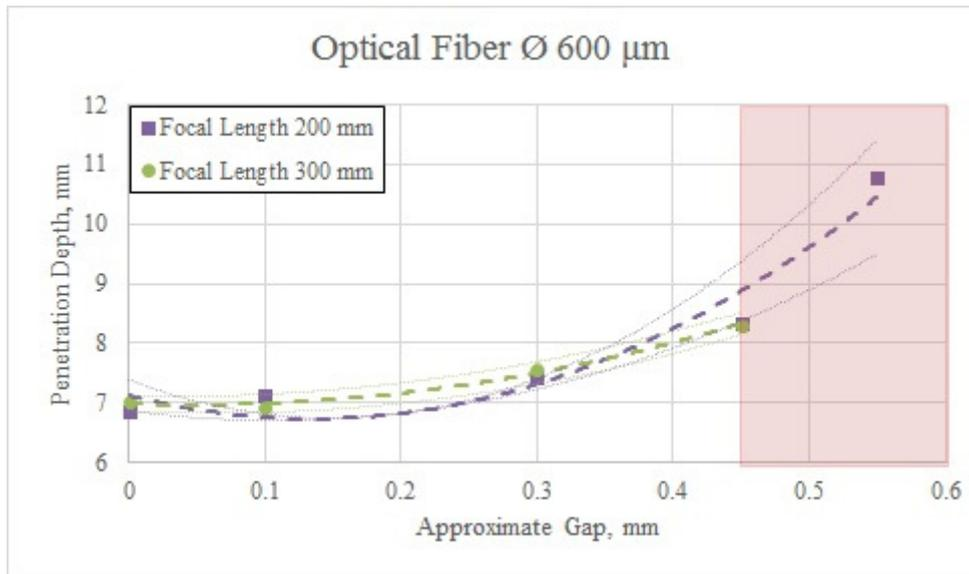
Fig. 2. Penetration depth of AH36 laser welds with optical fiber diameter 600  $\mu\text{m}$  and welding heads of focal length of 200 and 300 mm with confidence intervals (0.95), zone of unacceptable quality is marked with red,  $t = 14$  mm,  $P_L = 5$  kW,  $V_w = 1$  m/min, fpp = -4 mm.
