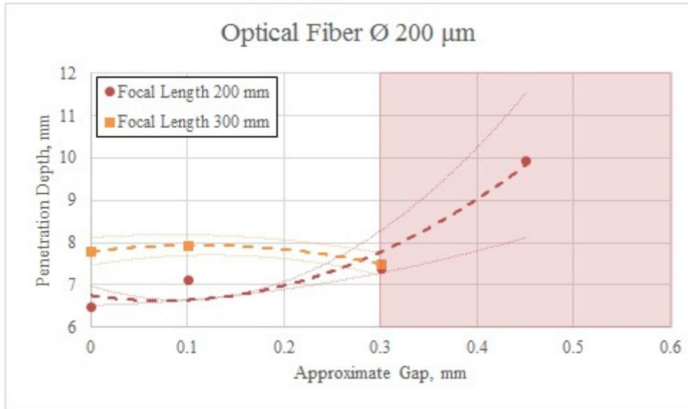
Fig. 1. Penetration depth of AH36 laser welds with optical fiber diameter 200  $\mu\text{m}$  and welding heads of focal length of 200 and 300 mm with confidence intervals (0.95), zone of unacceptable quality is marked with red,  $t = 14$  mm,  $P_L = 5$  kW,  $V_w = 1$  m/min, fpp = -4 mm.
