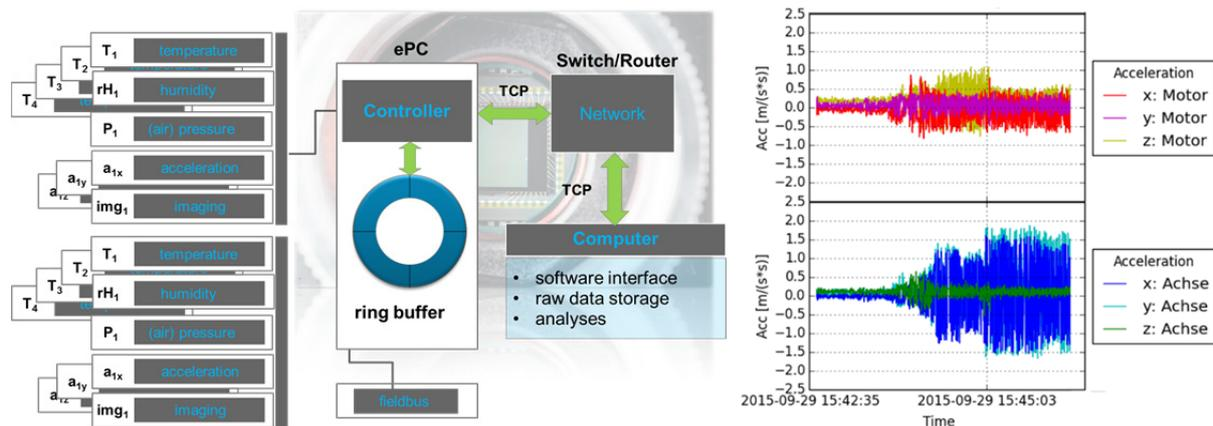
Fig. 1. (a) sensor grid architecture with embedded PC and network interface and paired peripheral sensors; (b) 3D acceleration plotting of vibrations during run-up of a high-speed drilling head for ultrafast laser machining.
