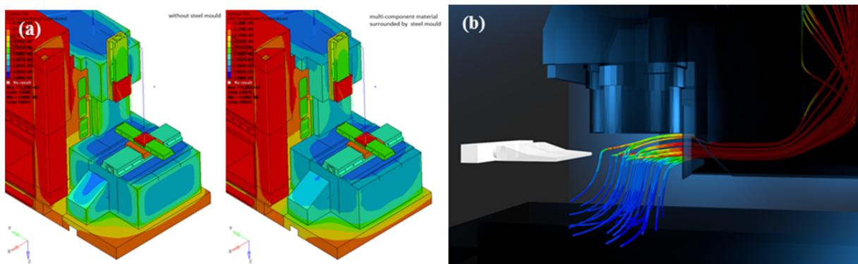
Fig. 2. (a) Temperature field after 1h heating by a change of the surrounding temperature by 2K. Comparative effect of the steel mould on the temperature of the components.  $T_{\text{parts}} [^{\circ}\text{C}] 20^{\circ}\text{C} - 22^{\circ}\text{C}$ ; (b) Pathlines of laser smoke particles blown by air nozzles and sucked by the suction system, integrated into the z-axis mounting bracket
