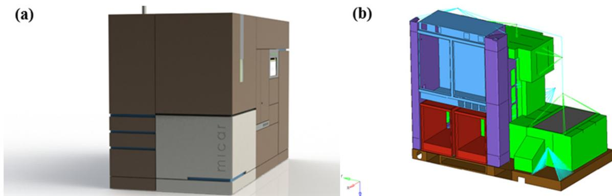
Fig. 3. (a) Ultrashort pulse laser machine C554.1 (b) modular machine platform of C554 with monolithic machine base, platform ground carrier, thermal isolated electrical compartment.
