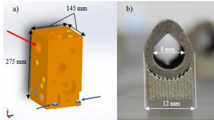
Fig. 2. a) Constraints of design b) Self-supporting pipe geometry.
