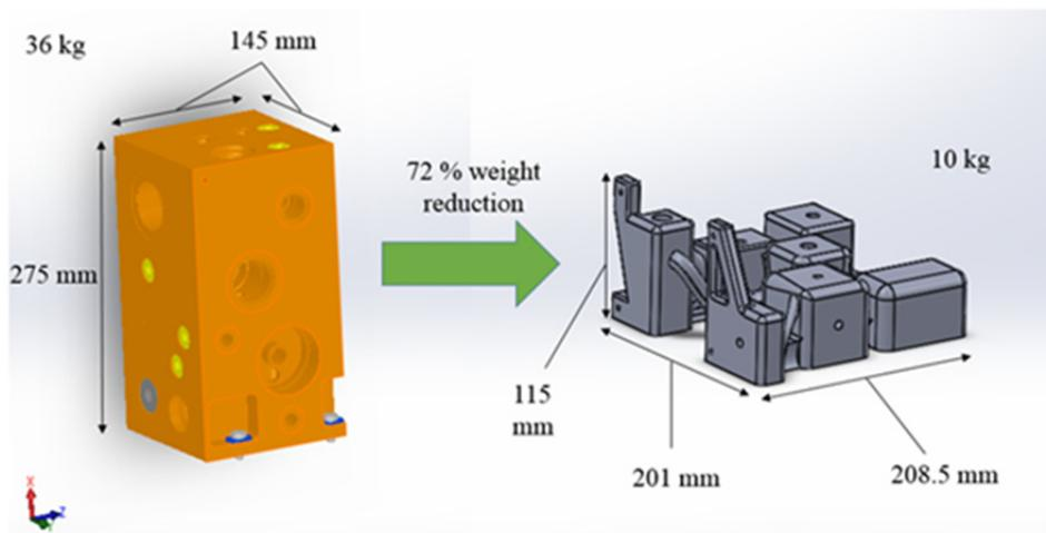
Fig. 3. Comparison between the old and the new model.
