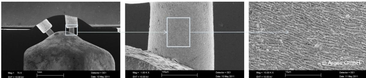
Fig. 3. (a) SEM image of the Cross section of a nozzle head with two injection nozzles; (b) Close-up of the negative tapered, fs-drilled hole; (c) Wall surface structure inside the hole.
