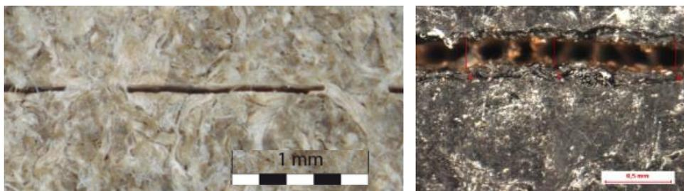
Fig. 4. (a) Genuine leather cut with fs laser at 0.5...1 m/s feed rate without any visible thermal damage; (b) Inevitable swelling of the genuine leather around the cut with longer pulse laser due to a larger heat affected zone.
