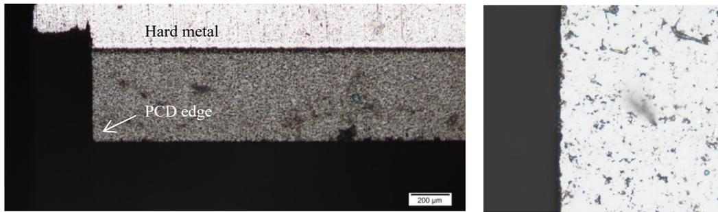
Fig. 8. (a) Microscope image of a cross section of the nanosecond laser machined PCD layer on hard metal; (b) Close-up of the PCD edge.
