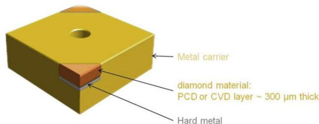
Fig. 7. Indexable insert with 2 diamond material tips.
