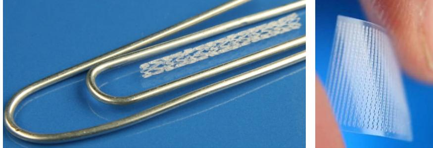
Fig. 5. (a) Stent made of bio-resorbable polymer; (b) Triangular sample geometry in PDLLA sheet for process optimization.
