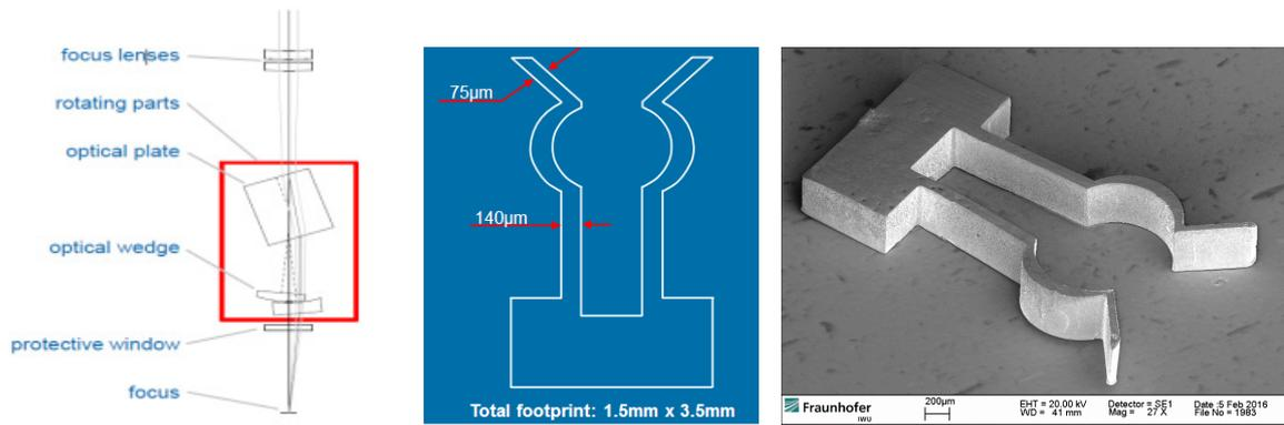
Fig. 2. (a) Optical setup of the trepanning head; (b) Dimensions of the CuBe micro clamp; (c) SEM image of the fs-machined micro clamp made of 500 µm thick CuBe sheet.
