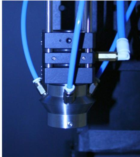
Fig. 4. Additive processing head for laser metal deposition: Coaxial powder nozzle, inlets for powder, carrier gas and shielding gas and focusing optics.
