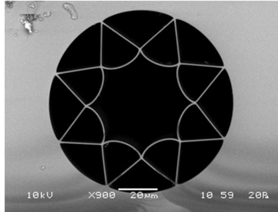
Fig. 2. Cross-section of a hollow core negative curvature fibre (NCF) with a core diameter of 42 $\mu\text{m}$ , suitable to deliver high average power ps and ns laser pulses in the near IR region.
