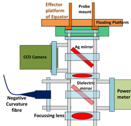
Fig. 3. Schematic of the processing head for ps and ns pulsed fibre delivered laser processing. The power meter and CCD camera enable closed-loop process monitoring and control.
