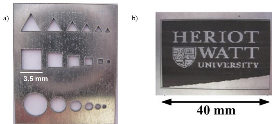
Fig. 5. NCF delivered nanosecond laser processing: a) cutting of  $0.3\ \text{mm}$  thick Aluminium at a scan speed of  $1\ \text{mm/s}$ , b) marking of Titanium at a scan speed of  $100\ \text{mm/s}$ .
