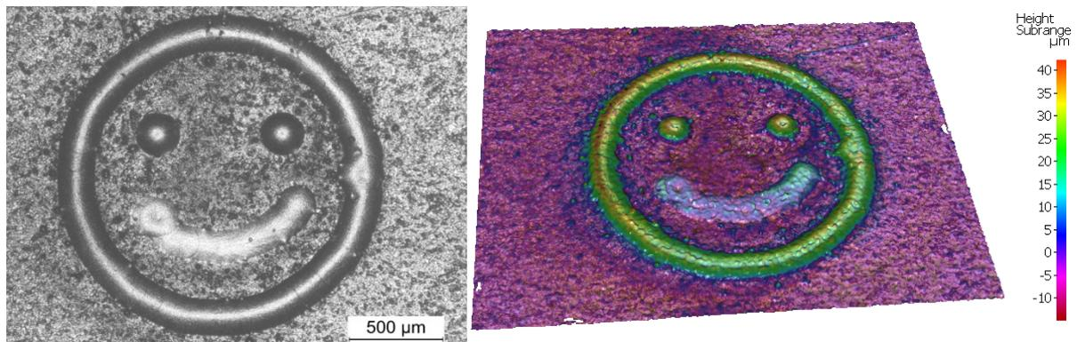
Fig. 6. Additively manufactured example of a “smiley face” from stainless steel 316 powder on SS 316 substrate. The height of the features is  $\sim 40 \mu\text{m}$ : a) shows the sample using a standard microscope. The surface profile in b) was measured using an ALICONA Profilometer.
